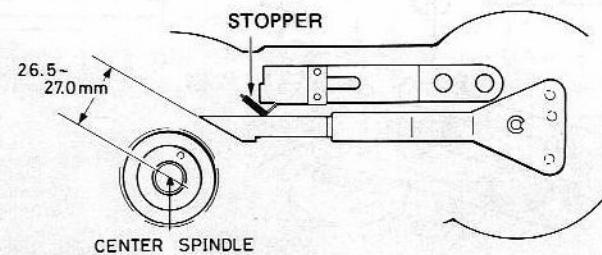
2. There is a shaft which is accessible with an ordinary screwdriver through the hole below the tonearm. When the stylus has reached a point approximately 55mm from the turntable center, turn the shaft clockwise or counter-clockwise and select a position where it actuates the auto-return.
